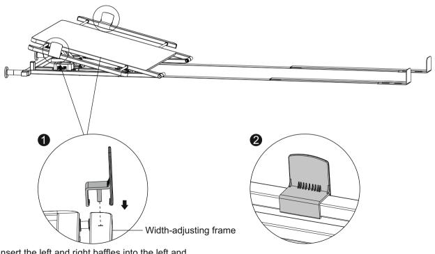
Insert the left and right baffles into the left and right square tubes on both sides of the bed frame, and insert the cylinder into the square tube hole.
