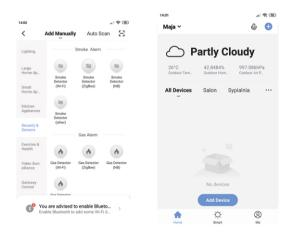
Install the battery to make the power on, press the button on the side of the device and hold on for 5 seconds to enter into the Wi-Fi configuration state (the red standby indicator flashes fast indicates that it is in the EZ mode configuration mode. If the indicator light flashes slowly, it indicates it is in the AP configuration mode). There are two modes displays in the APP interface which can be switched to each other before configuration start. As below:
